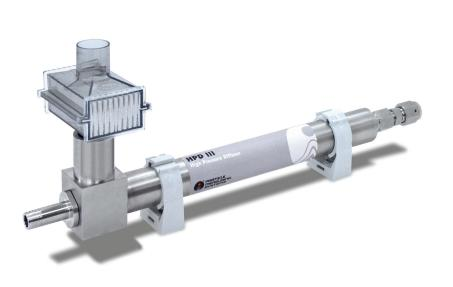
Sampling gases at pressures greater than sea level, such as 40 – 100 psi, is challenging for some particle counters. Connecting pressurized air or gas to a particle counter can defeat its flow-metering system. High Pressure Diffusers (HPDs) have been developed to correct this problem. HPDs reduce the pressure of the gas to about that of sea level by allowing some of the air/gas to diffuse and allow the particle counter's flow-metering system to function as designed.
